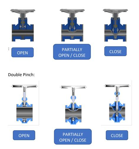
For sizes from DN150, two pinch rods driven by the torque or thrust applied by the actuator push the sleeve both from the top and also from the bottom to the closed position. When opening, the pinch rods simply retreats back and the elastomer, the pinch rods simply retreats back and the elastomer sleeve recovers its normal position (also helped by the line pressure)
